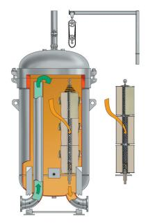
Typical Clay Treater Housing Flow Diagram (Including optional items)
